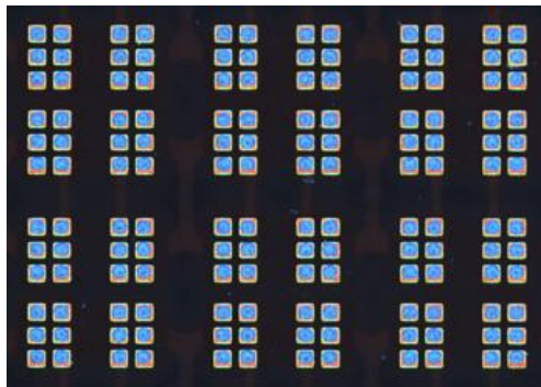
LED锡膏印刷检测
